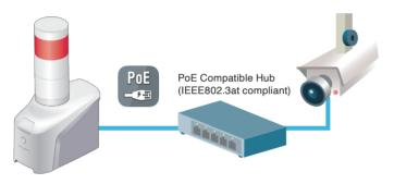
This model has the NHV-D features plus PoE power capability. It can be used in areas where it is difficult to secure power or to facilitate network camera connection. (IEEE802.3at compliant)
